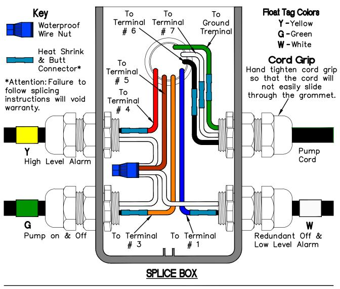
Control Panel Series Float Function Color Code Splice Box Model Drawing No.
